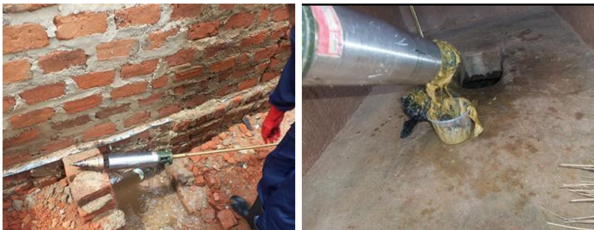
Figure 2. Sampling of faecal sludge: Pit sludge sampler (Left)-; Pit sludge sampler in action (Right).
